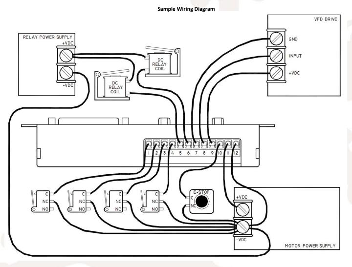
Please note that all connections shows above are optional except for the power supply and E-Stop switch. A few frequently asked questions for wiring are below:
